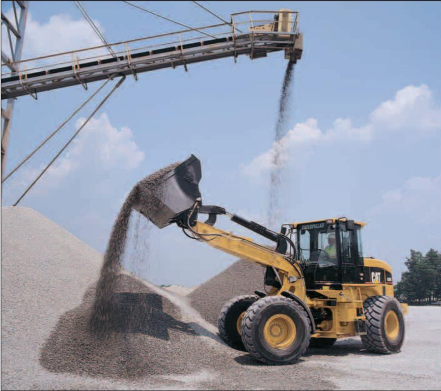
**Linkage Design.** Versatility is the key benefit of the VersaLink loader linkage. The 930G can be configured in many ways:
