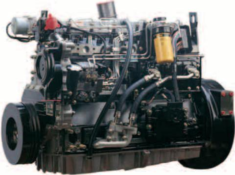
**Caterpillar Engine.** The six-cylinder, 3056E direct injection, turbocharged (DIT) engine with air-to-air after cooler (ATAAC) has a proven reputation for reliability, durability and performance. Fuel injection is electronically controlled for precise timing.
